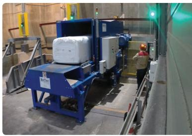
In the RDF thermal power station, the trapping materials and fiber sludge acummulated in the paper mill as well as various municipal and commercial waste from external delivery are thermally recycled.
