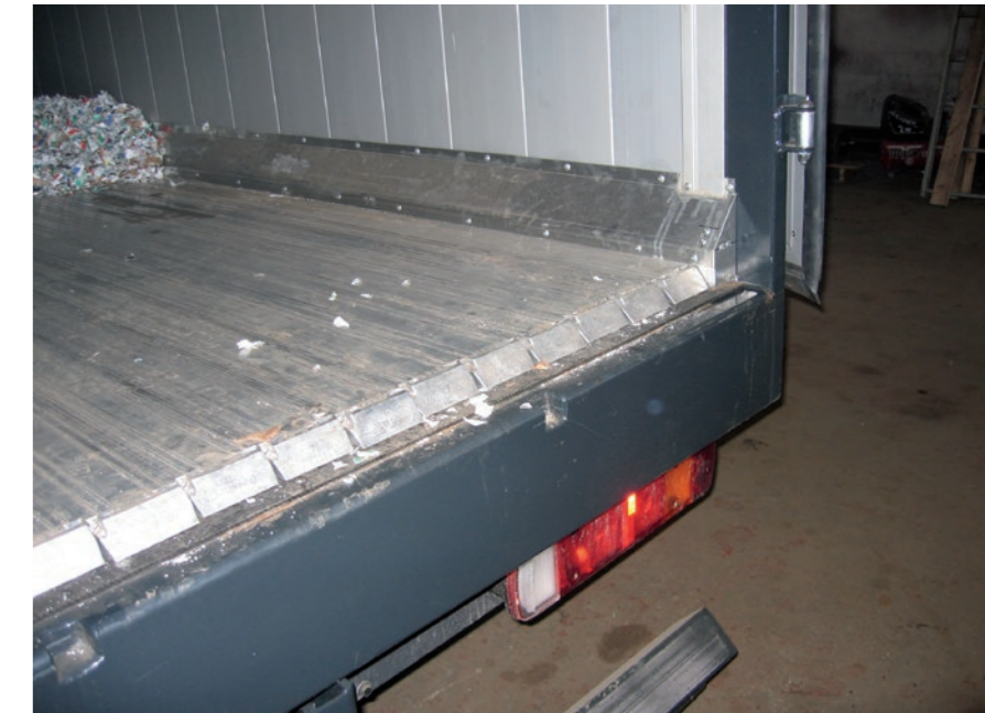
Unloading backwards with a Walking Floor.
