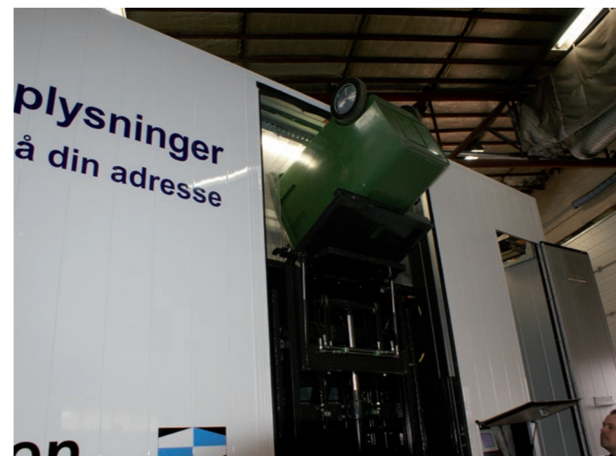
Feeding via bin lifter with weighing system for standard bins up to 660 l.
