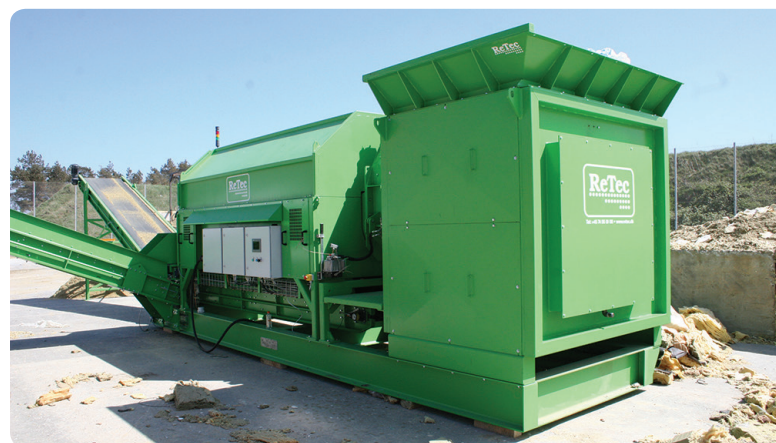
ReTec mineral wool recycler is built on a practical frame so it can be easily moved
