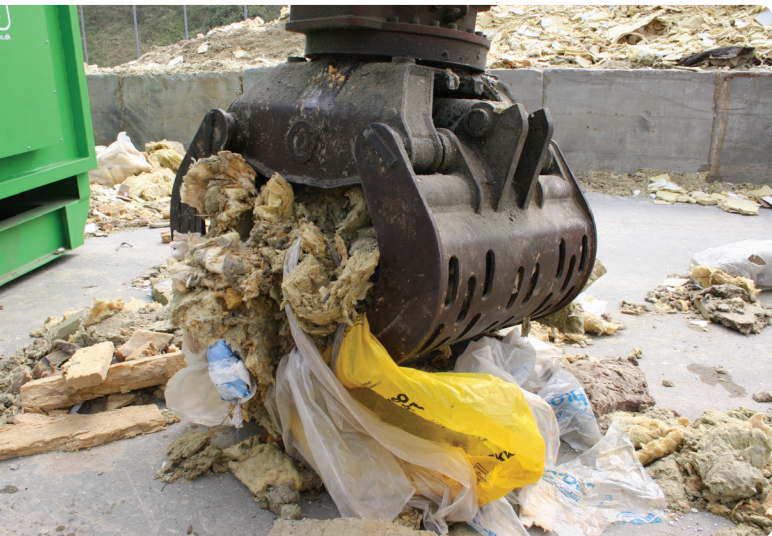
Input material, a mixture of wrapping, stone wool, glass wool, foam, rubber, nails, screws, wood and much more. Only mineral wool and material, smaller than the size of the sieve dimension will be released in the final fine fraction.
