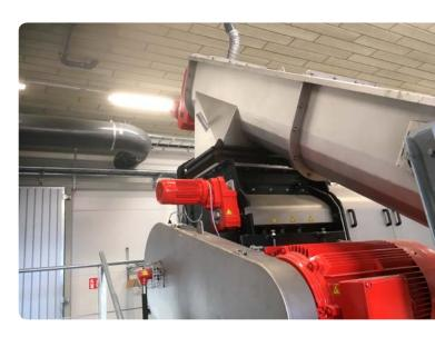
ration in the incinerator, while the remaining organic material is broken up by being flung up against a screen. Water and/or liquid fat waste is then added as a lubricant, so that it forms the so-called "slurry".
